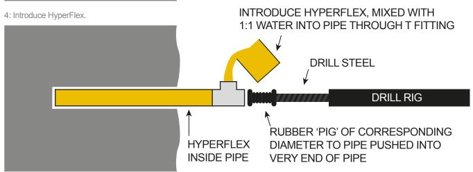
5: Using a drill rig with a 'Pig' of corresponding diameter attached to the end of the drill steel, push the pig forward the entire length of the pipe. This will force the grout out of the end of the pipe and force it back towards the rock face, filling the annulus area.
