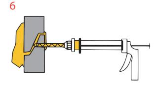
Pump gun vigorously to expel grout to refusal or seal. If grout is washing out, either pump slower or stop pumping and watch grout until it reacts halfway down the mixer then quickly give a pump to expel and repeat.
