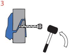
Tap the mixer with the nut on it into the hole until snug.
