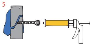
Quickly align threads on the tubes with the nut on the miser and tighten until secure.
