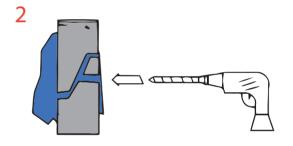
Drill 5/8" diameter hole to intersect the leak path.
