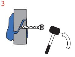
Tap the mixer with the nut on it into the hole until snug.
